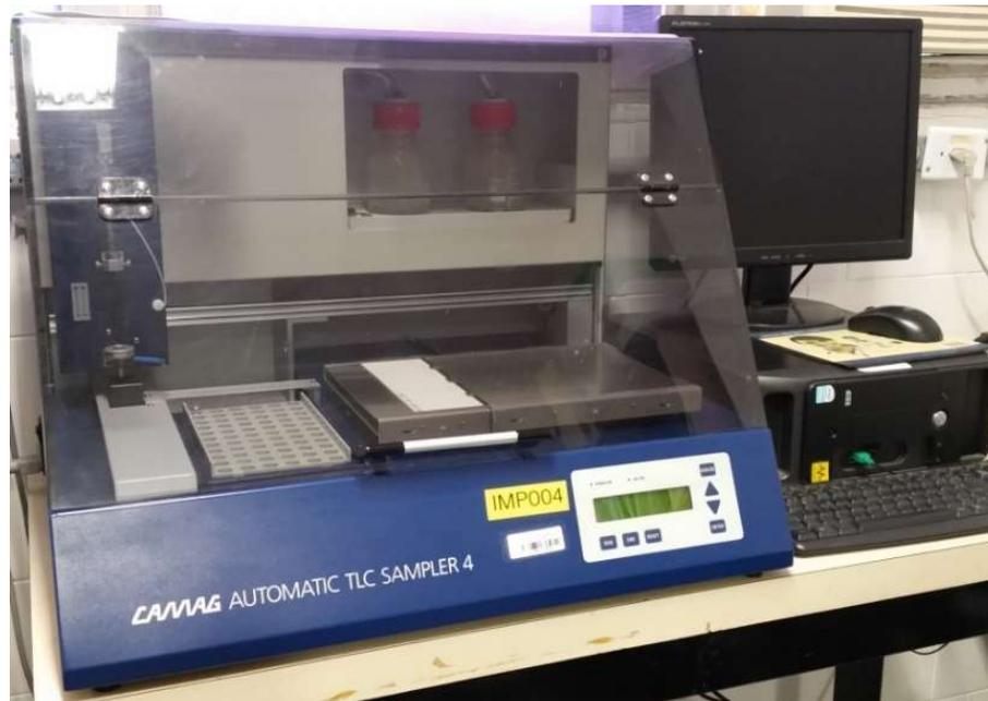
Figura 4.3 – CAMAG Automatic TLC Sampler 4.
