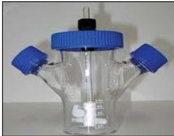
Figura 1.3: Frasco Spinner (fonte: Tri Stars Laboratory Glassware & Scientific Equipment)
